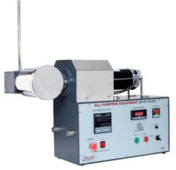
Ball mills can be used for crystalline material. A ball mill is useful for mixing dry materials and under certain conditions wet material. The ball mill jar is made of complete stainless steel 304. The diameter of S. S.ball varying between 10 mm to 30 mm is provided with a ball mill. The ball mill can be attached to the main drive through the universal gearbox.
