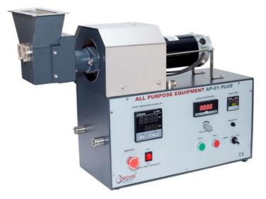
It is used to granulate tablet slugs and pellets. Two power drive rollers with teeth force the material against breaking combs. The dry granulator can be directly attached to main drive.
