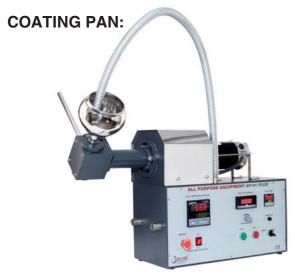
A coating pan is used for coating tablets. The coating Pan can be mounted on the main drive at any angle up to 45 ° through the universal gearbox
