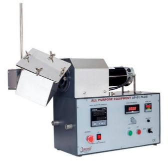
The Cube mixer is based on a movement, which through its tumbling effect produces a homogeneous mixture in the shortest time possible. The powders to be mixed are treated very gently. The cube mixer can be attached to the drive easily through universal gear box. The mixing rods are made of S. S. 304 with diameter of 10 mm.
