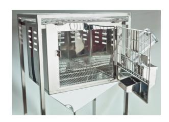
Orchid's metabolic cages for large rodents are equipped with system for separation of feces and urine. Each system is divided in 3 parts- cage body, separation hopper and feed- water supplying unit.
