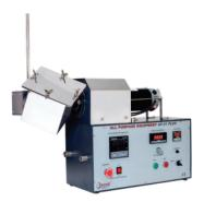
The Cube mixer is based on a movement, which through its tumbling effect produces a homogeneous mixture in the shortest time possible. The powders to be mixed are treated very gently. The cube mixer can be attached to the drive easily through universal gear box. The mixing rods are made of S. S. 304 with diameter of 10 mm.
