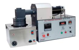
This mixer is designed to be used for mixing for pastes, ointments & creams in vessel which is jacketed by heating elements to maintain the temperature of material inside vessel thermostatically. It can also be used for wet powders. This mixer is provided with a mixing paddle & scrapper, which is shaped in such manner so that there is minimum clearance with the mixing kettle. This unit is suitable for attaching directly to main drive
