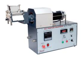
This attachment is used in the preparation of ointments, salves, pastes, dough and similar products. The rolling action is produced by three hard S. S. rollers, which are 120 mm long and 42 mm diameter. The roller mill can be directly attached to the main drive.
