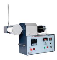
Ball mill can be used for crystalline material. Ball mill is useful for mixing drymaterials and under certain conditions wet material. The ball milljar is made of complete stainless steel 304. The diameter of S. S.ball varying between 10 mm to 30 mm are provided with ball mill. Ball mill can be attached to main drive through universal gear box.
