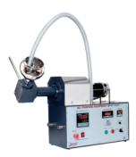
Coating pan is used for coating tablets. Coating Pan can be mounted on the main drive at any angle up to 45° through universal gear box.
